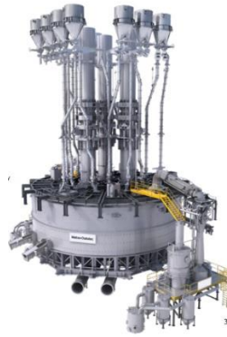
Figure 6. Metso Outotec submerged arc furnace.
