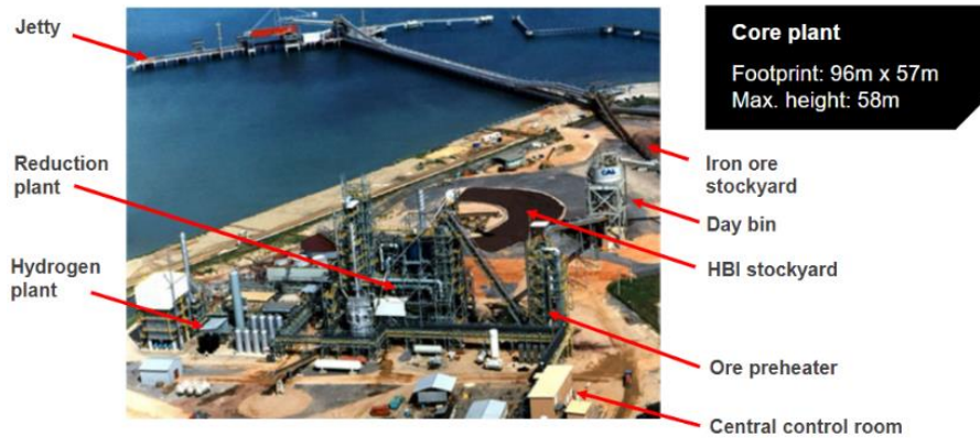
Figure 7. Aerial view of Metso Outotec’s Hydrogen driven circulating fluid bed iron ore reduction plant built in Trinidad.
